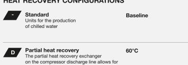
Hot water to be used to produce DHW or combined with air handling units (AHU)
