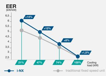
The increase in efficiency compared to similar fixed speed units is expressed by drawing the EER trend to the conditions defined by the ErP directive 2009/125 / EC necessary for the calculation of SEER seasonal parameters.
