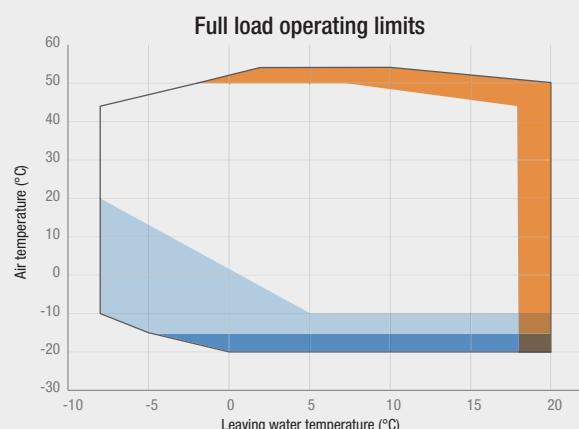
The diagram shows the operating limits of versions /E, /SL-E. For versions /K, /SL-K, the max outdoor temperature is lowered by 4°C. For versions /CA, /SL-CA, the max outdoor temperature is lowered by 2°C.
