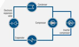
The two compressors are combined in the same refrigerant circuit, ensuring higher efficiency values at partial loads in comparison with a proposal with units with independent circuits.
