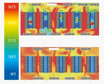
The image above shows an excellent example of the advantages in terms of hot and cold flow separation obtained through aisle containment.
