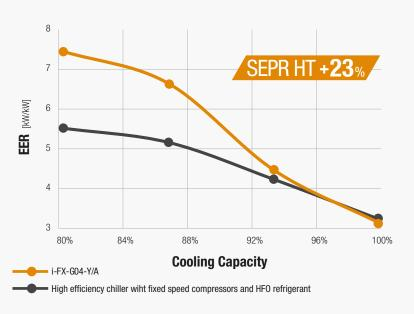
The increase in efficiency compared to high efficiency ErP 2018 compliant fixed speed units is expressed by drawing the EER trend to the conditions defined by the ErP directive 2009/125 /EC necessary for the calculation of SEPR HT seasonal parameters.
