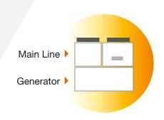
Redundancy increases uptime. i-FX-G04-Y extends this concept also to the electrical supply: the unit, equipped with an ATS\*, can be connected to two separate power lines to enhance the system's dependability.
