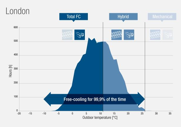
Graphics above show the cumulative hours per year of a unit working 24/7 in either Mechanical, Hybrid or Total free-cooling. Operating water temperature (in/out) 22°C/20°C.
