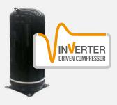
The DC INVERTER technology, applied to compressors, allows for the modulation of the refrigeration power based on the real necessities, continually varying the speed of the compressor rotation, notably heightening the efficiency at partial loads.
