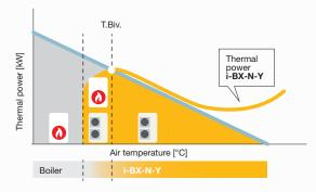
The auxiliary sources are used to meet the energy demand at low outdoor temperatures by integrating the heating capacity of the heat pump.
