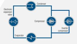
The two compressors are combined on the same refrigerant circuit, ensuring higher efficiency values at partial loads in comparison with units with independent circuits.
