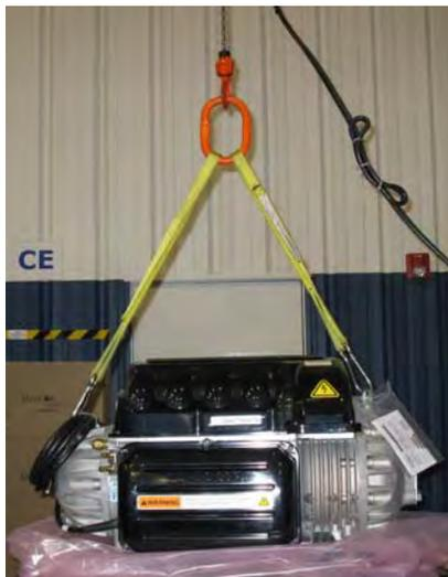
Figure 8 Configuration de levage
